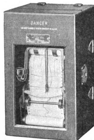
HIGH-VOLTAGE TYPE U AMMETER
